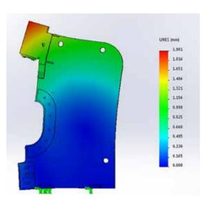
Deratech machines are built with a few tons extra steel. The extra weight is not the big production cost, but ensures stability and robustness. It results in reliable and accurate machines with a long service life. All frames and parts are calculated for strength and deflection with "finite elements" method.
