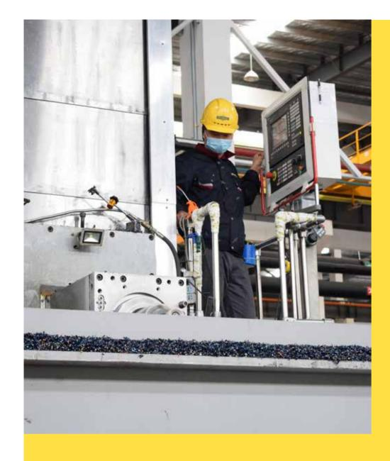
Frames are milled in one go on brand-new CNC milling machines.
